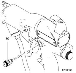
Figure 2 Fan Air Adjustment Valve
