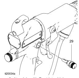
Figure 3 Atomizing Air Restrictor Valve
