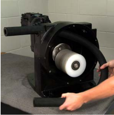
Figure 9 Roller in 6 O'Clock Position
