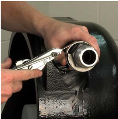
Figure 10 Tighten the Clamp
