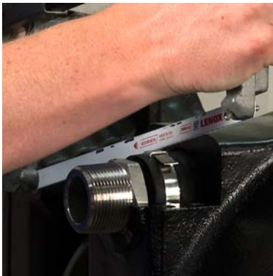
Figure 2 Cut the Clamp
