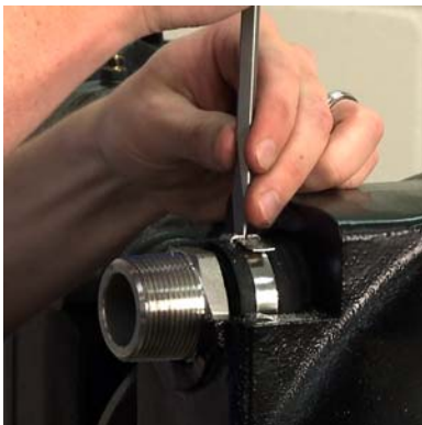
Figure 3 Remove the Clamp
