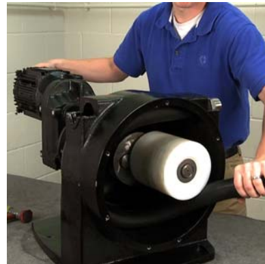
Figure 4 Roller in 3 O'Clock Position
