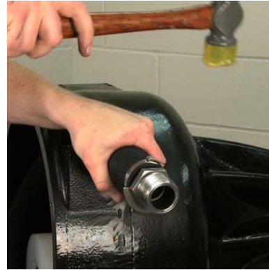
Figure 11 Seat the Barbed Fitting
