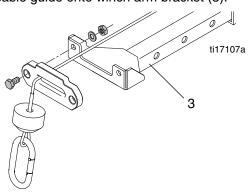
4. Slide winch arm bracket (3) into winch arm (2) and secure into place by tightening extension clamp (15) and inserting the safety pin.
