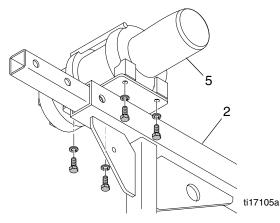
3. Use bolts, washers, and nuts (supplied) to assemble cable guide onto winch arm bracket (3).
