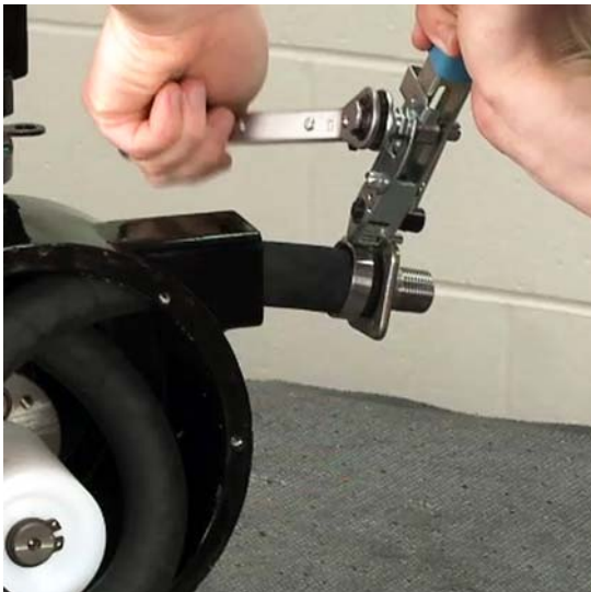
Figure 10 Tighten the Clamp
