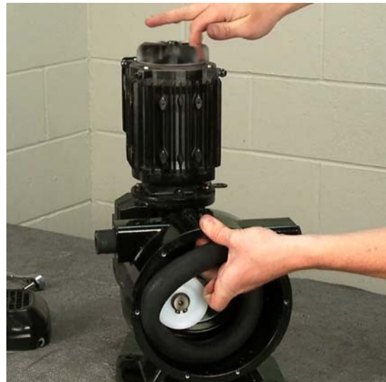
Figure 4 Roller in 9 O'Clock Position
