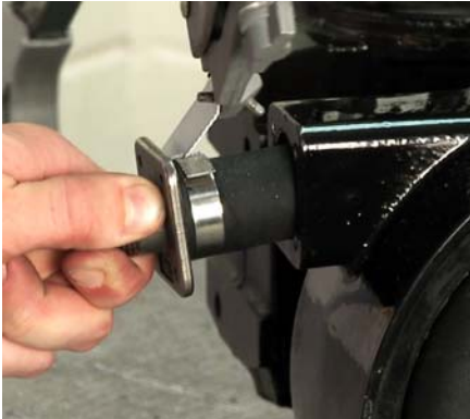
Figure 2 Cut the Clamp
