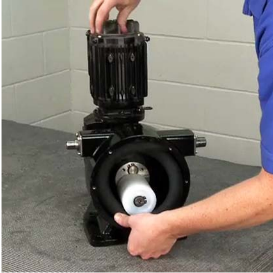
Figure 9 Roller in 6 O'Clock Position
